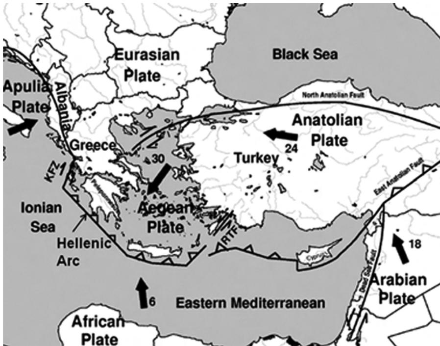
Fig. 1. Schematic illustration of the principal movements affecting active tectonics in the Greek Aegean and the eastern Mediterranean. Thick arrows indicate the direction of the motion relative to Eurasia. The values ( $\text{mm yr}^{-1}$ ) are shown near each arrow (Source: McClusky et al. 2000.)
